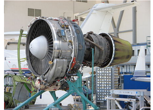
An ALF 502 geared turbofan from a Bombardier Challenger 600
